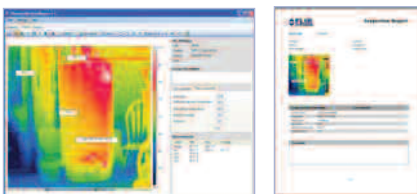
QuickReport™ PC software enables user to analyze Temperature of all thermal pixels of any FLIR Camera JPEG images
