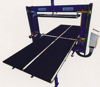
THE WINTECH OSCILLATING BLADE CONTOUR CUTTER
